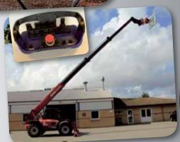
As Sky Lifter is radio-controlled, there are no limits to working height. The range of the remote control is 100 metres.
